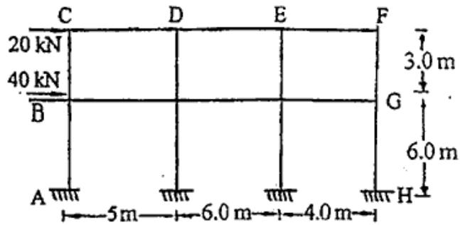
8. Analyse the continuous beam as shown in Fig. by stiffness matrix method and plot B.M.D.
